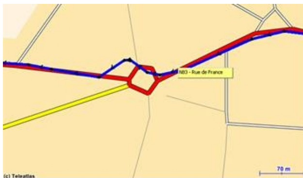
Inaccuracy of the recorded track points at a 70m zoom level
