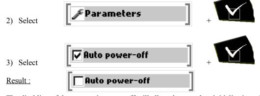
The disabling of the automatic power off will allow the complete initialisation of the RoadMaster GPS.
